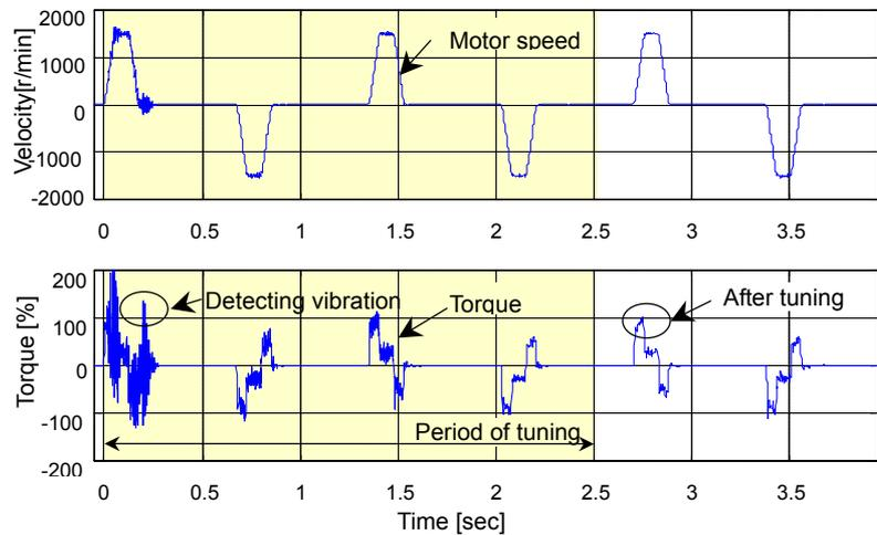
machine-analyzer data and writes the optimized parameters to the amplifier. These operations are semi-automated and easy to check its effectiveness.
