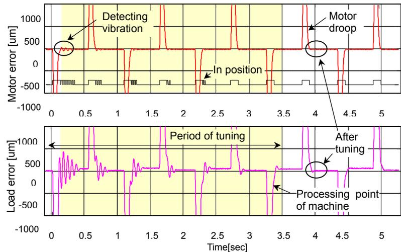
During the course of the tuning, the residual vibration is gradually suppressed at each movement. The machine should be operated for several cycles consecutively because the tuning ends when the controller determines that the residual vibration has become small. After tuning, the servo suppresses the motion of both motor and load.
